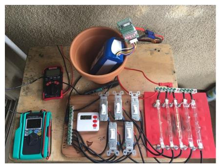
I first install the blinky to balance the battery and to keep it relatively balanced during the discharge routine. I make sure that the multimeter is reading voltage and I have written my target voltages on the board. For a 6S battery this is 6 X 3.8 or 22.8 volts DC.
