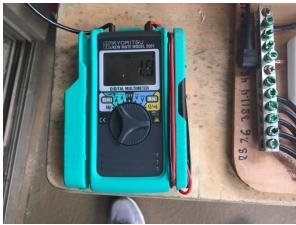
Next, I switch loads on, one at a time and keep an eye on how much current is flowing. When all five lights were on the load was about 7.2 amps, roughly a discharge rate of 1.44C, well within the capability of the battery. Incidentally the battery did not get warm. Total discharge time was about 14 minutes. I set the timer for 9 minutes, then 3 then 2.
